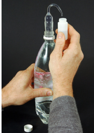
Figure 18: Photo of the glass nozzle fitted to the PET bottle as used when displacing mineral oil to the scintillation vial (adapted from Leaney and Herczeg, 2006)
