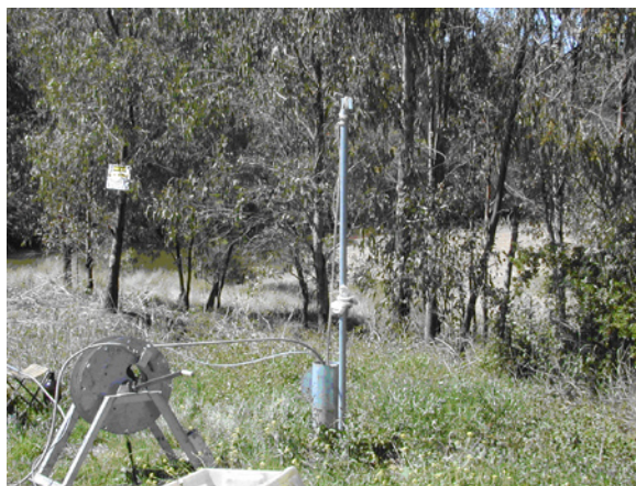
Figure 10: Groundwater sampling in a monitoring bore using a pump
