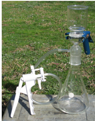
Figure 16: Hand operated vacuum pump filtration unit
