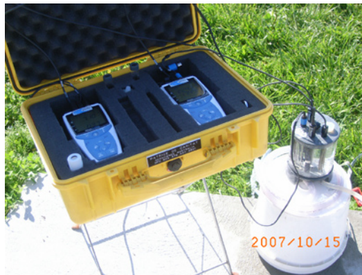
Figure 13: Testing of field measurements using multiparameter meters
