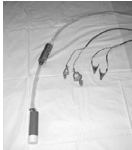
Figure 9: Submersible 12 volt pump
