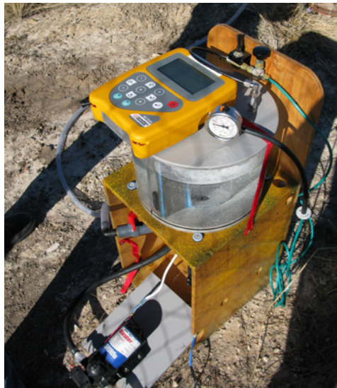
Figure 22: Setup of gas separator and field gas analyser
